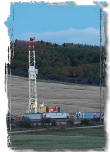
A service rig. Courtesy of Canadian Association of Oil Well Drilling Contractors.
